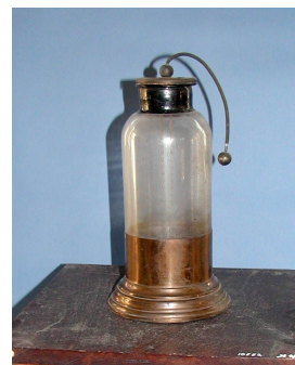
Illustration 1: A Leyden jar is a primitive version of a capacitor.
