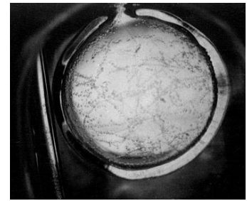
Illustration 3: A hydrogen bubble chamber image.
