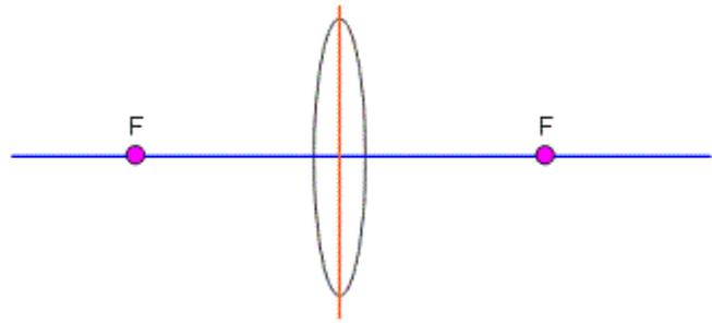
Illustration 1: Diagram showing a double convex lens.
