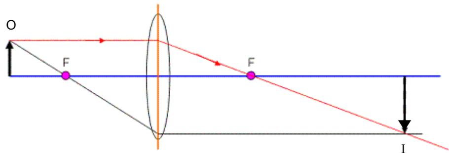
Illustration 3: Rule 2 is parallel to the principle axis.
