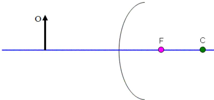
**Diverging** mirrors are so named because the light rays that are reflected off the mirror go apart (diverge) on the real side.
