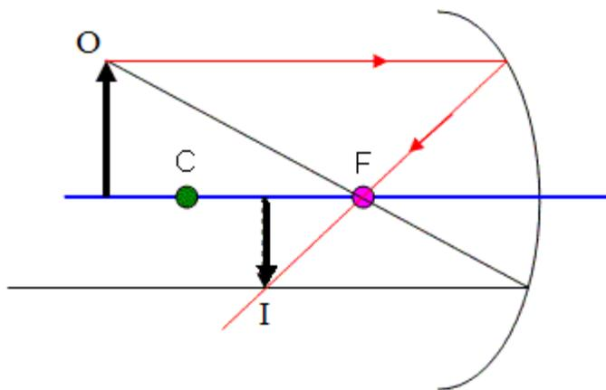
**Converging** mirrors are so named because the light rays that are reflected off the mirror come together (converge) on the real side. It's ok to call these mirrors either converging or concave.
