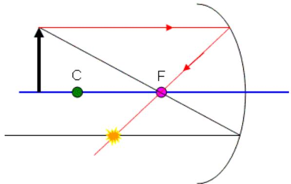
Illustration 9: Light Ray parallel to the principle axis.
