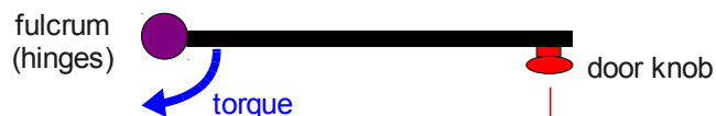
Illustration 1: The torque is quite large when the force is applied far away from the fulcrum.
