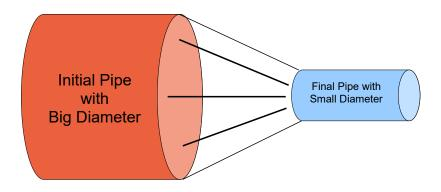
Volume Flow Rate<sub>1</sub> = Volume Flow Rate<sub>2</sub>
