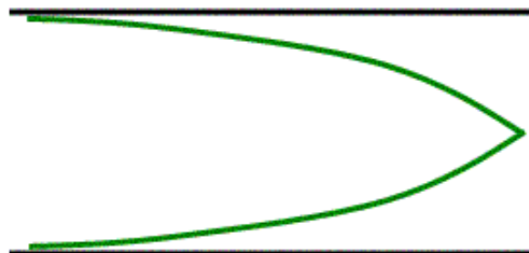
Illustration 8: Fundamental for a closed tube, showing reflection.
